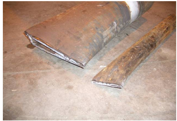
Fig.10 – Sheared 194 mm (7-5/8 in) casing with 76 mm (3 in) liner pipe removed from the test piece.
