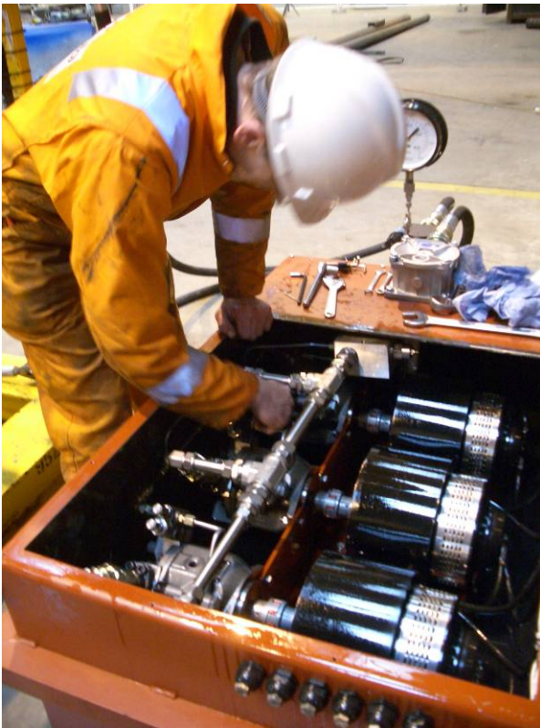
Figure 7 – DC Motor Pumps in SCM Pod
